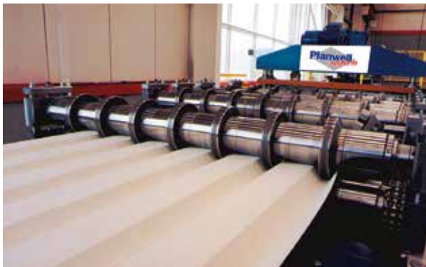
Inside the Planwell factory, manufacturing Permaroof Metal Roof Sheeting
